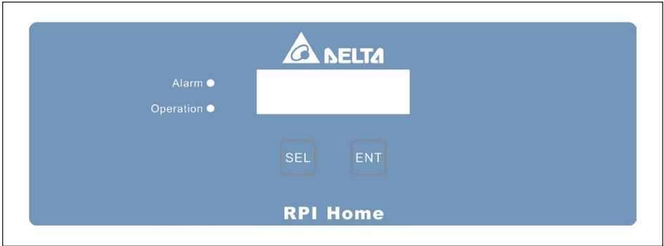
**Figure 3-3 : LCD display and buttons**
